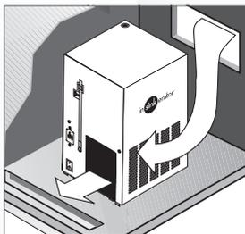
It is recommended to have your cabinetry vented to create adequate air-flow for the NeoChiller to work to its optimum.
