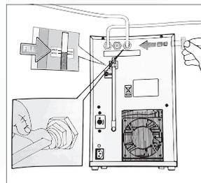
**IMPORTANT NOTICE:** Remove red pug from ICE BANK FILL port (C). Connect plastic tube to this port on the other end to the Y fitting (smaller side). Turn on water supply and fill ice bank use fill marking. When full remove plastic tube from chiller and insert plug.
