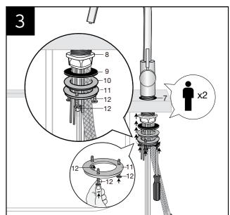
\* NOTICE: Property Damage. Do not pinch or break copper tubing. Do not distort the last 25 mm (1") of tubing.
