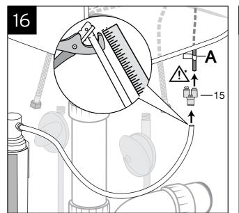
\* NOTICE: Property Damage. Do not extend the lines farther than the 400 mm (16") provided. Ensure tube(s) and "Y" connector fit securely.
