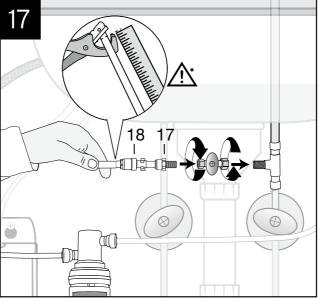
\* NOTICE: Property Damage. Tube runs need to form to the cabinet's contours to allow storage space with no sharp bends. Tubes need clean, perpendicular, burrfree cuts to ensure a true fit. Join remaining tube to cold water supply only.
